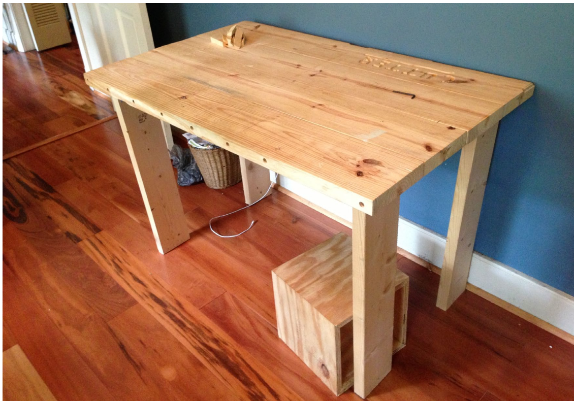
My first prototype wooden desk. Learned how to glue boards together and drill dowel holes. Without aprons, it wobbled.
