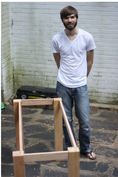
The final base. The left apron is on the inside because it will have a ledge to hold all the cords in the back.
