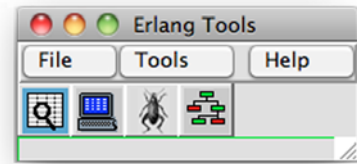
Figure 5.15 The Erlang Toolbar. This is handy if you often start TV, Pman, Debugger, or Appmon. It's even possible to add your own custom tool icons to the toolbar.
