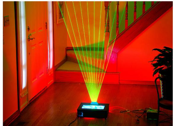
**Figure 17:** A Laser Harp, an Arduino-based musical instrument made of light. Photo taken from [Hobley 2010].
