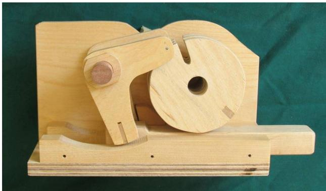
This view with the back panel removed better illustrates how the lock opens. The L-shaped part on the left turns clockwise to open the lock. This pulls the bolt (on the bottom) back to the left at the same time.
