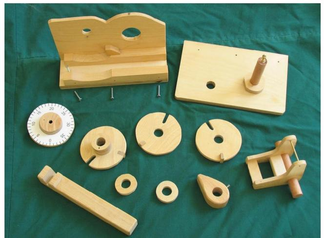
And here's the lock disassembled, showing all of its parts. Really, there is not very much to it. Note that the shaft that the rotors turn on is glued into the back piece of the plywood. This shaft itself doesn't turn. The rotors are semi-loose on this shaft. Ideally, they would turn with a bit of friction so they wouldn't overshoot with momentum when dialing a combination quickly.
