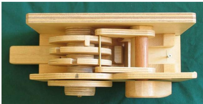
Like most real combination locks such as a Dudley or master Combination locks, the core of this lock consists of three rotors. Each rotor has a notch in it, and
