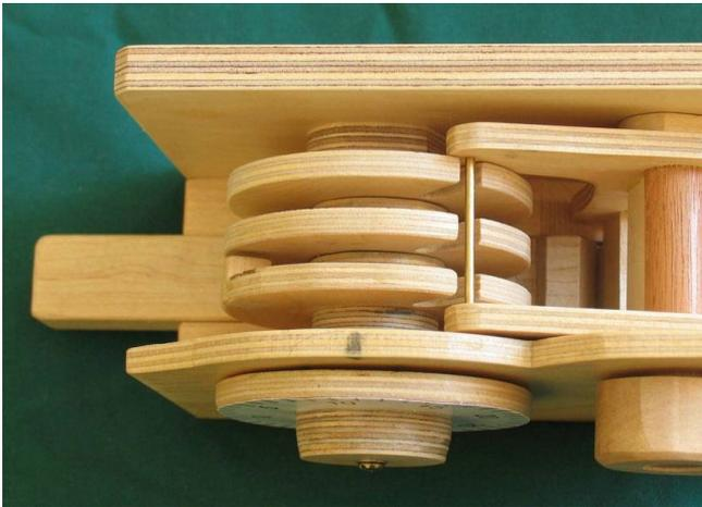
After that, the rotation is again reversed, now turning clockwise again until the notch in the front most rotor is lined up with the bar. The picture at left shows all three notches lined up. The lock is ready to open.
